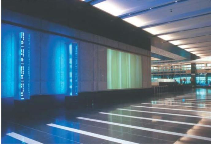
▲ **Figure 7-8** Fiber-optics, dichroic glasses and LEDs were used by James Carpenter Design Associates in this lobby installation for Bear Stearns in New York. The green zone is produced with fiber-optics and dichroic glass, it serves as a soft contrast to the moving blue LED information screens. (James Carpenter)
