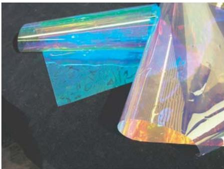
▲ **Figure 1-5** Radiant color film. The color of the transmitted or reflected light depends upon the vantage point. Observers at different places would see different colors (see Chapter 6)
