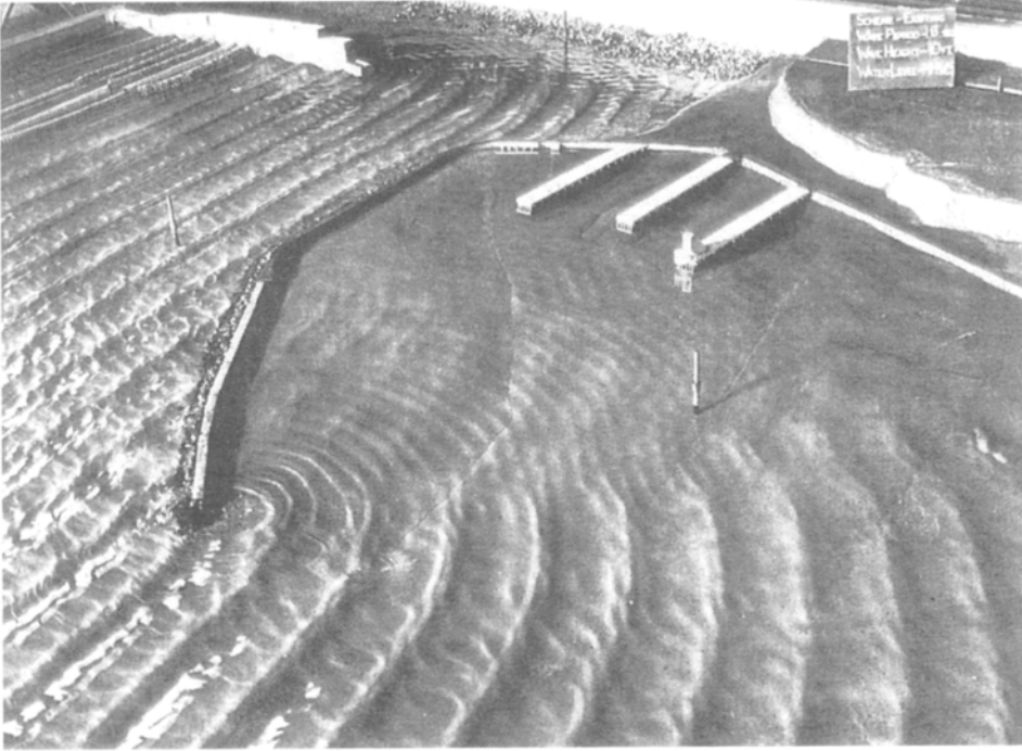
Fig. 2.10 Diffraction of water waves by a breakwater. Reproduced with permission of Arnold Publishers and HMSO from Newton, R.E.I. (1990) Wave Physics . Edward Arnold, London.
