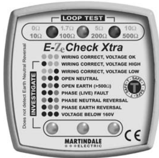
Figure 2.9 Earth loop impedance socket tester (courtesy of Martindale-Electric).
