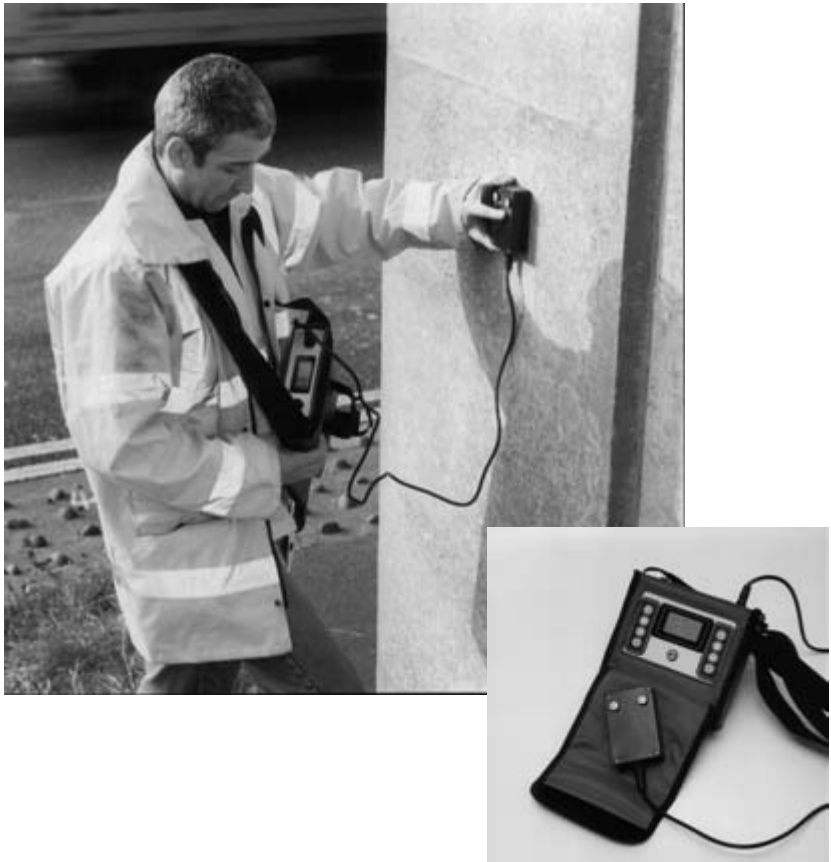
Figure 2.7 Reinforcement cover meter (courtesy of CMT Instruments).
