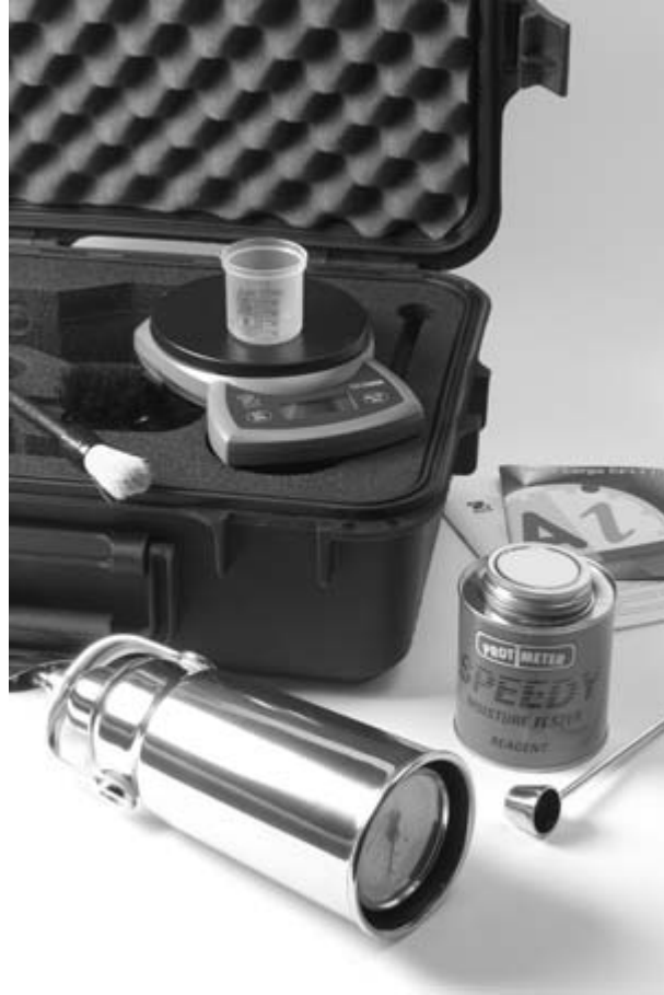
Figure 2.8 'Speedy' calcium carbide moisture meter (courtesy of Protimeter Ltd).
