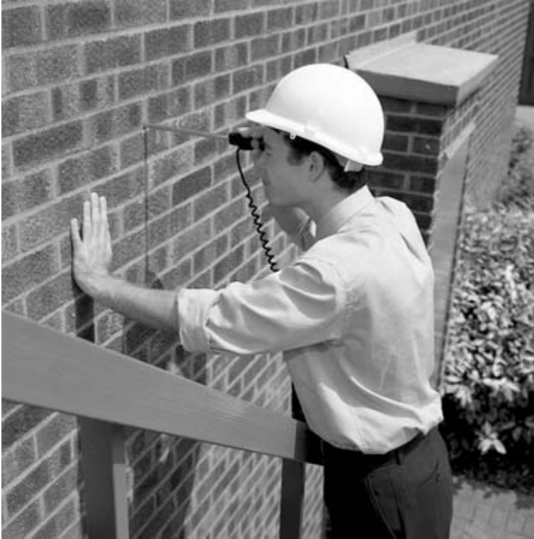
Figure 2.5 Surveyor using a borescope (courtesy of Olympus Industrial).
