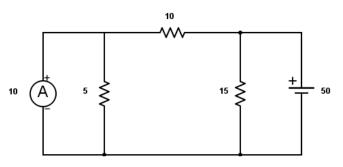
Determine the maximum power that can be transferred to a load resistance connected across 10  $\Omega$ .
