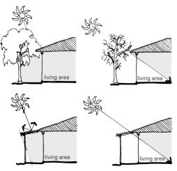
With ideal north orientation sun can be excluded in summer and admitted in winter using simple horizontal devices, including eaves. For situations where ideal orientation cannot be achieved (eg existing house, challenging site) it is still possible to find effective shading solutions. [See: Passive Solar Heating: Orientation]
