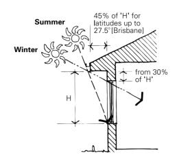
The general 'rule of thumb' for calculating eaves width is given above. This rule applies to all latitudes south of and including 27.5°S (Brisbane, Geraldton). Within this range the rule is self adjusting - going south winter sun angles decrease, but at the same time the need for solar access increases as climates becomes cooler.
