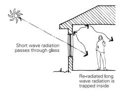
Radiant heat from the sun passes through glass and is absorbed by building elements and furnishings, which then re-radiate it. Re-radiated heat has a different wavelength and cannot pass back out through the glass as easily. In most climates, 'trapping' radiant heat is desirable for winter heating but must be avoided in summer. Shading of wall and roof surfaces is important to reduce summer heat gain, particularly if they are dark coloured and/or heavyweight.
