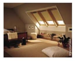
The 'right size' of skylight admits just enough light for the job and no more. Several methods exist for helping to decide on the size and spacing of skylights. WERS for Skylights provides an energy rating system. The scheme takes account of key differences between the energy performance of windows and skylights and the differing responses of houses to these building elements.
