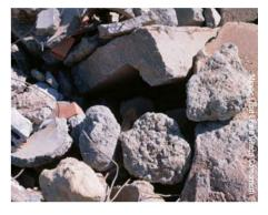
Break remnants into small pieces before final set to allow later use as backfill or recycling.
