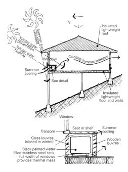
The above system is a cost effective solution for achieving high thermal mass passive design with the high insulation levels and low embodied energy of lightweight construction for difficult sites.
