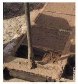
At its simplest, mud brick making involves placing mud in moulds which, after initial drying, are removed to allow the bricks to dry slowly (not in direct sun). Moulds can be made from timber or metal – anything that can be shaped to provide the desired size for the bricks.
