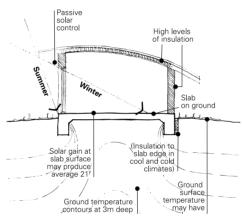
Earth coupling allows the floor slab of a well insulated house to achieve the same temperature as the earth a few metres below the ground surface, where temperatures are more stable (cooler in summer, warmer in winter). In winter, added solar gain boosts the surface temperature of the slab to a very comfortable level.
