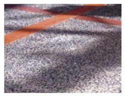
Abrasive blasting of the concrete surface will also provide varied effects.
