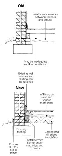
These slabs can be either suspended on the original subfloor walls and footings, or if the old floor is close to ground they can be an
