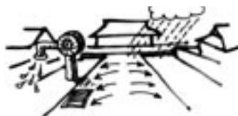
A pump to take up stormwater
