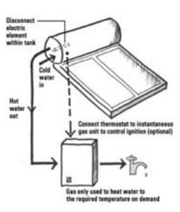
The electric element has been removed from the solar hot water service to reduce greenhouse gas emissions. The solar hot water service and the instantaneous gas unit have been connected in series so that gas is only used to boost water temperature when it is actually required. [See: Hot Water Service; Solar Hot Water]
