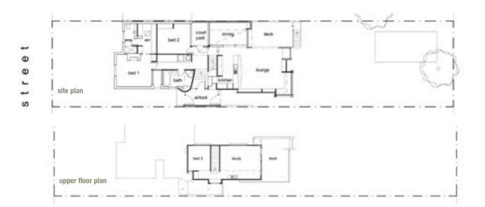
Courtyards were located to the north of the building to maximize solar gain, with an extensive area of double glazing in the roof over the dining/ living area. [See: Passive Solar Heating]
