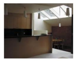
For night lighting, surface-mounted and pendant lights were selected exclusively, to eliminate holes in the insulation necessitated by low voltage transformers. 98 percent of lights have energy efficient compact fluorescent or circular fluorescent globes. [See: Lighting; Insulation installation]
