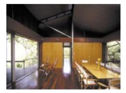
The house was designed to be built from modular components, fabricated off site and transported to site by barge for erection. A 900mm modular design allowed standard material sizes to be used throughout. This reduced costs and minimised wastage in construction. All plywood and aluminium paneling was made to a 900mm wide grid to minimise any waste at the factory and to ensure that there was no site waste generated from construction.
