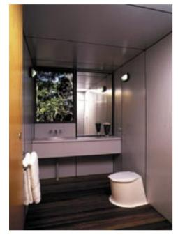
toilet system (Rotaloo) that has two pans arranged back to back in the two bathrooms. The system is commercially available and allows for up to two pans and provides a system of composting bins that may be rotated when full to allow full composting before it is removed for use in the garden. The dry residue has nil health risk if composted properly. The system has Australia wide health department approval. [See: Waterless Toilets]
