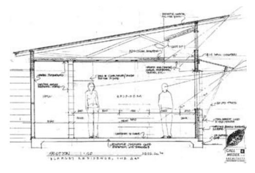
The external walls of the house are insulated, using a polyester/cotton material to R1.5. The comparatively small window/door glazed area ensures maximum possible wall insulation. This is cheaper than double glazing.
