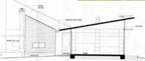
rooms. The kitchen/living/dining area and bedrooms are grouped into separate "mini houses" with a courtyard between each. All these rooms face north for maximum passive solar gain. Behind these, on the south side, are three "pods" containing two bathrooms and a carport storage area. [See: Orientation, Passive Solar Heating]
