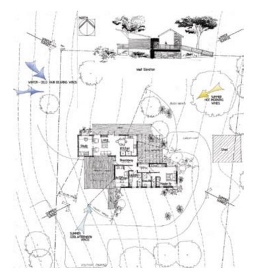
Once these decisions have been made, auxiliary heating and cooling strategies are worked out, and a decision is made about what sort of solar hot water heater to use. Numerical values are determined for glass area on the north, south, east and west walls, total thermal mass in cubic metres, minimum insulation levels in the roof, floor and walls, and the size of the solar hot water system. Finally, a five-stage designers checklist is followed to execute the design.ii
