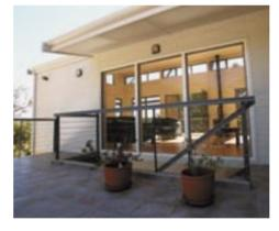
The windows are placed to take advantage of the sea breeze from the south-west. The house can be divided into 'breeze ways' to channel air through whatever part of the house most needs cooling, including to the north the living wing, to the east into the sleeping wing, and straight through onto the solar deck at the northeast of the house.
